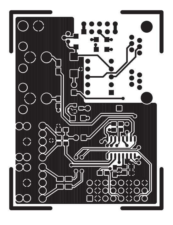
Figure 6. Si3000DC-EVB Component Side
